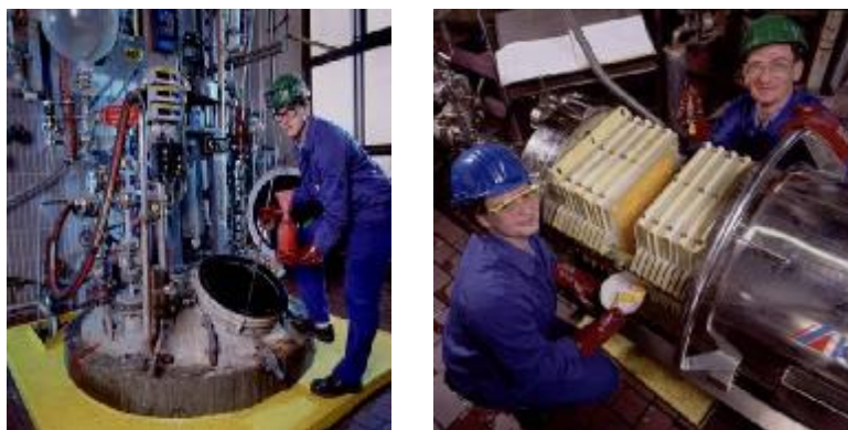
Figure 2: Continuously stirred tank reactor for coupling-reaction of an azo-pigment and filter press used for separating pigment press cake from coupling suspension.
