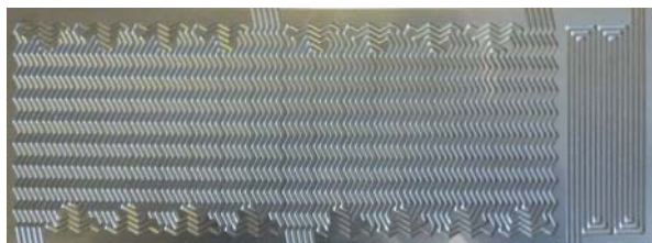
Fig. 5. Multistream plate with Straight and Wavy channels.
