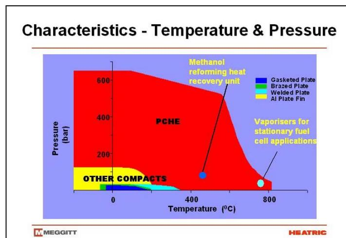
For fuel cell vehicle applications, the heat transfer system must also be lightweight, as well as compact, and comprise a minimum number of components. With headers and nozzles attached to the PCHE cores, the complete heat exchangers are highly compact, typically comprising about one-fifth the size and weight of conventional heat exchangers for the same thermal duty and pressure drops. This is attributable to:
