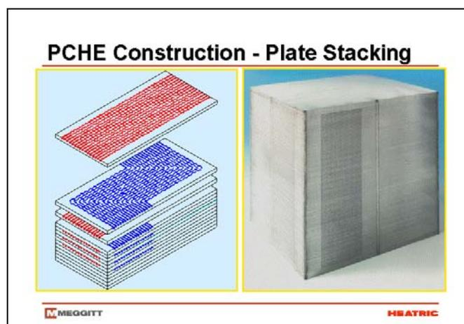
Diffusion bonding is a high temperature solid state joining process that promotes grain growth across the metal boundaries, resulting in a joint exhibiting parent metal strength and ductility.
