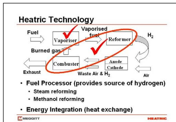
We presented a concept incorporating 20 reactions stages and 11 heat exchangers into a single reforming/pre-reforming module at the AIChE 2002 Spring Meeting (Johnston and Haynes, 2002). This novel and innovative application of Printed Circuit Technology permits the number of individual components to be dramatically reduced, with follow-on manufacturing cost savings. The same principle can be applied to methanol reforming (Johnston et al. 2001).
