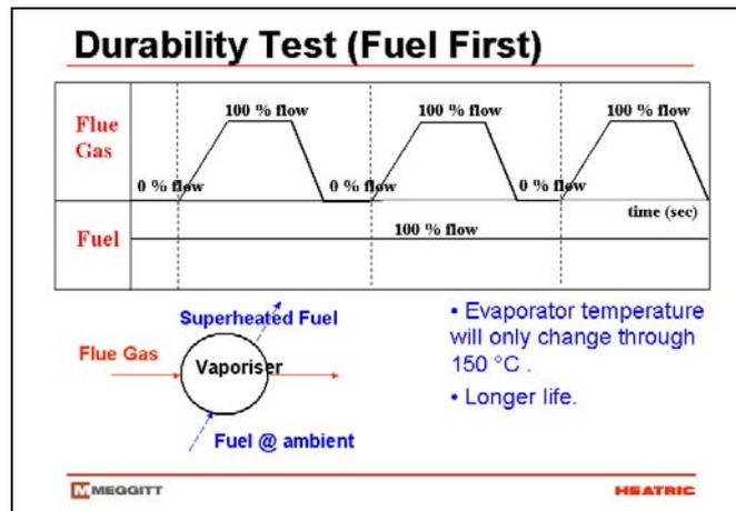
Another issue concerning temperature change within the vaporiser is unstable boiling. The nature of unstable boiling has been well reported: the main design challenge is to overcome the rate of temperature change caused by an unstable saturation line.
