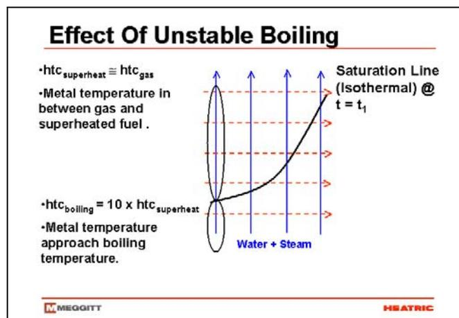
One way to overcome this problem is to design the vaporiser to operate co-currently. In this way the maximum temperature change that may be caused by unstable boiling is minimised.
