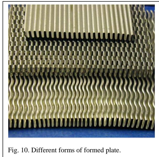
In addition to Heatric's traditional method of passage forming, photo chemical machining (also called chemical milling), alternative processes have been developed to address the challenge associated with high temperature materials including electro-chemical machining and formed plate construction. Formed plate (FPHE) is a diffusion bonded plate fin derivative.
