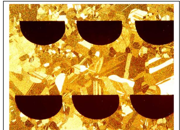
Fig. 2. Micrograph of section through diffusion diffusion bonded PCHE core
