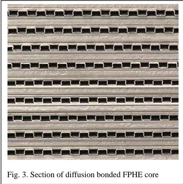
Fig. 3. Section of diffusion bonded FPHE core
