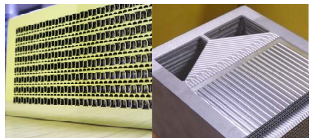
Fig. 3. H 2 X sections: cross-layer, with corrugated fins and etched plates in alternating layers (left); in-layer, with corrugated fins and etched plates in the same layer (right).
