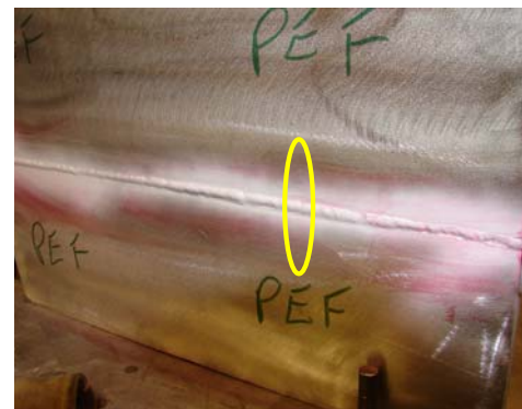
Fig. 7. Welded plates, showing indicative area from which tensiles specimen would have been prepared.
