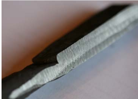
Fig. 4. Forge welded steel piece [3].
