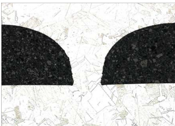
Fig. 5. Micro showing grain pattern at a diffusion bonded joint (section taken through a PCHE).
