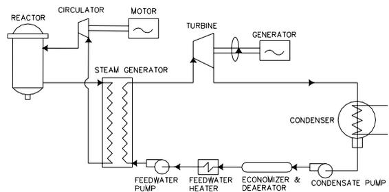
The medium temperature indirect gas turbine cycle (MHTGR) offers some increase in efficiency up to 38%. The major weak point is the steam generator. The low heat transfer coefficients of helium when compared with water leads to the need for large steam generation units.
