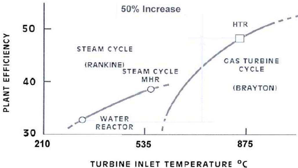
There are variants on the gas cooled reactor, for instance both GT-MHR and PBMR use the direct gas turbine cycle. The current GT-MHR concept has a reactor using conventional fuel and all of the rotating equipment associated with the power conversion system is on a single shaft. PBMR has a less conventional pebble bed reactor and the rotating equipment is split between three separate shafts.
