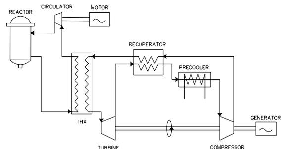
High temperature gas reactors have the unique ability to use the Brayton cycle. With the single phase Brayton cycle efficiencies of 48% can be easily achieved.
