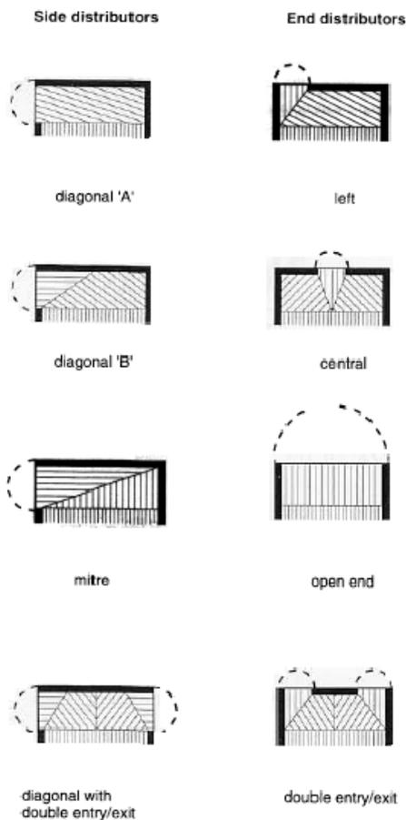
Typically with this type of exchanger the distributor is a relatively small proportion of the plate, 20% or less. The Ingersoll-Rand plate fin also uses a distribution system.
