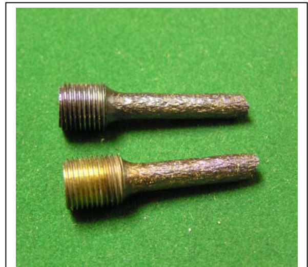
Fig. 8. Tensile sample for diffusion bonded alloy 617 showing necked region.
