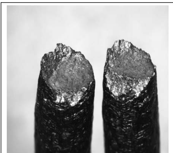
Fig. 7. Fracture surface of a diffusion bonded alloy 617 tensile sample showing cup-and-cone fracture.
